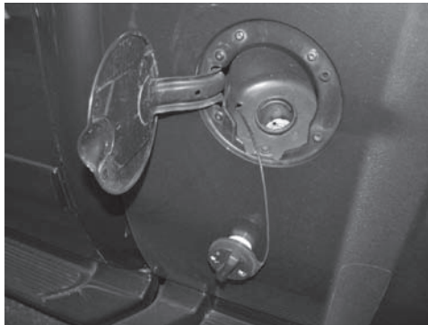
Figure 10.8 Gasoline filler tube that is only designed to fit unleaded gas pump nozzle.
